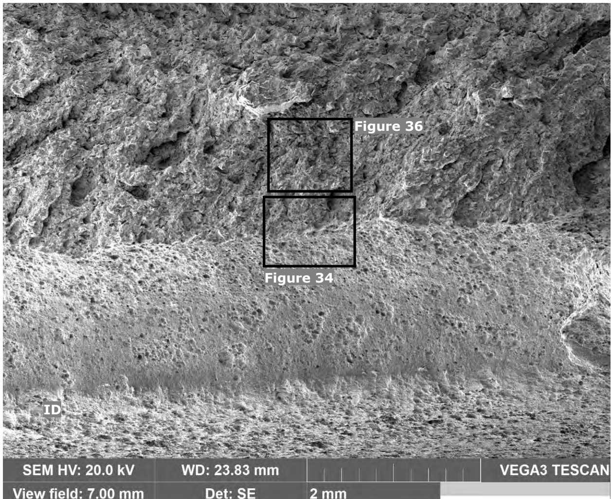
Figure 33. SEM image of Sample S2 adjacent to the ID surface; area indicated in Figure 32.
