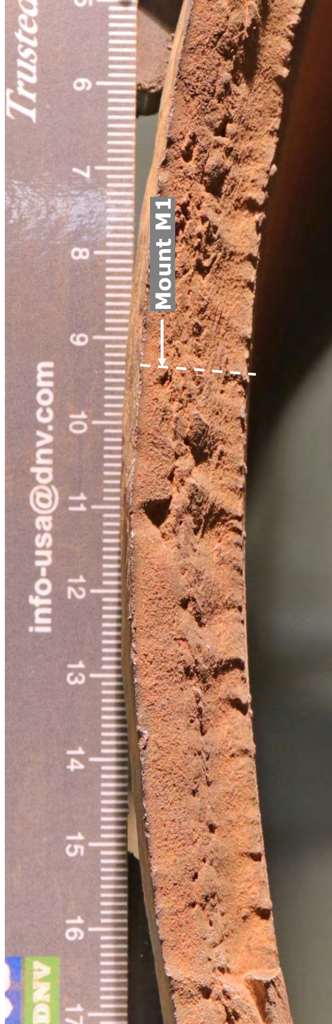
Figure 20. Photograph of the fracture surface of PS A between the 12 and 1 o'clock orientations. Units of ruler are in cm. Flow direction is into the photograph.
