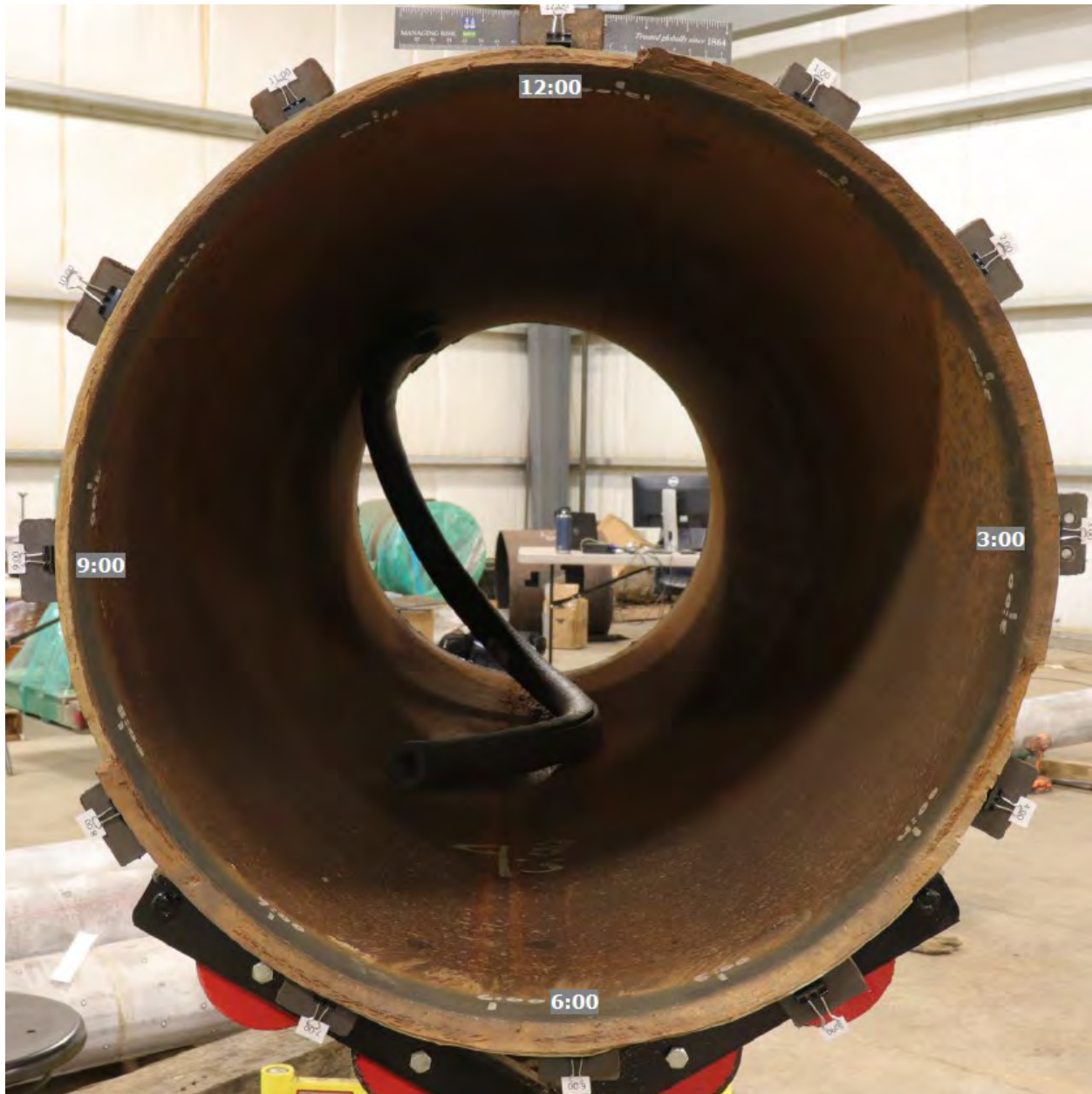
Figure 15. PS A Fracture Surface (Upstream to Downstream)
