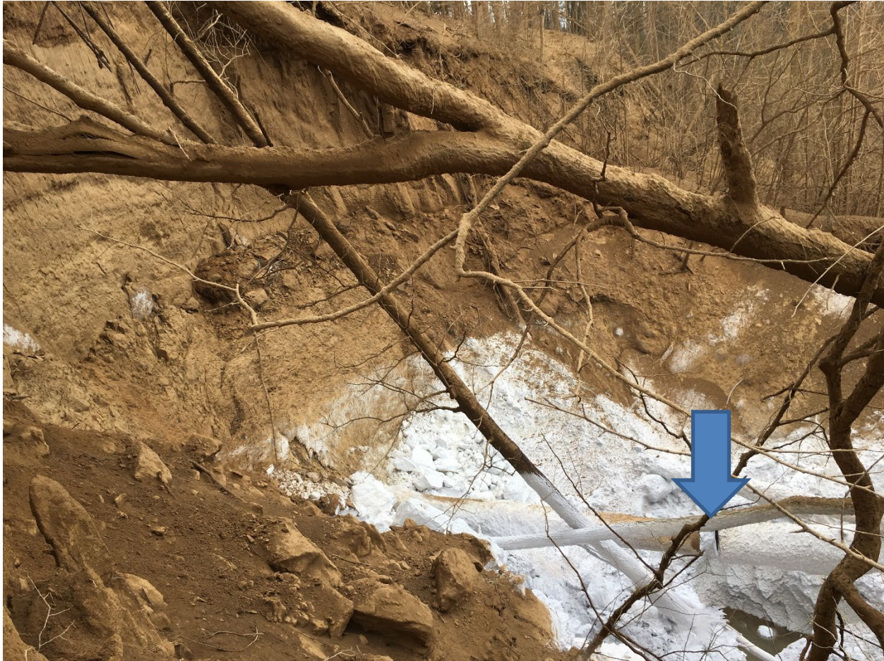
Figure 3: Crater Created by the Rupture Containing Fallen Debris (dry ice, and the failed pipe sections) (Blue Arrow is Pointing at the Pipeline Separation)
