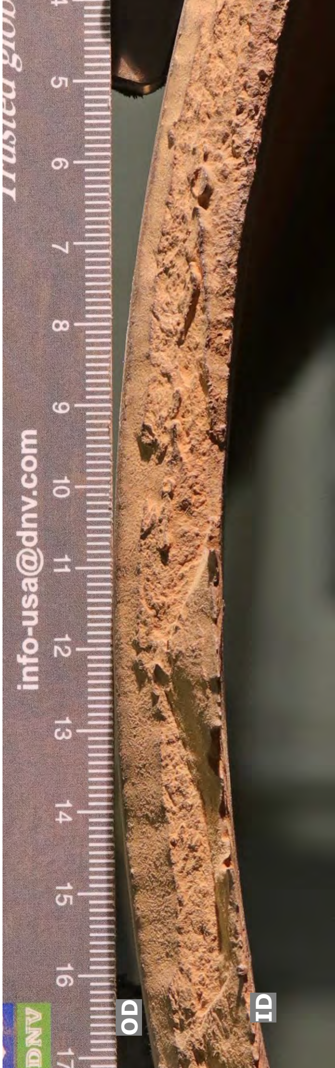
Figure 28. Photograph of the fracture surface of PS A between the 8 and 9 o'clock orientations. Units of ruler are in cm. Flow direction is into the photograph
